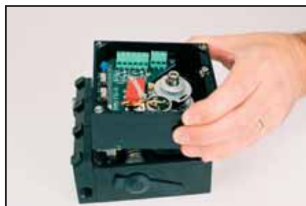
Place F5 unit on top, tighten screws
