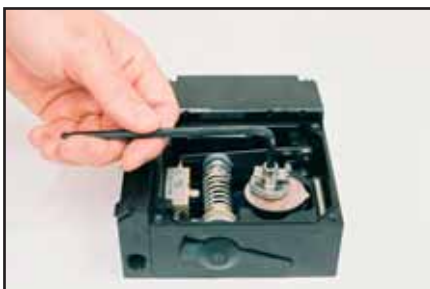
Install coupling on P5/EP5
